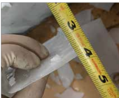
The Night Scan Powerlite IQ was tested at -15° F (-26° C) with a 1/4" (6mm) of ice
